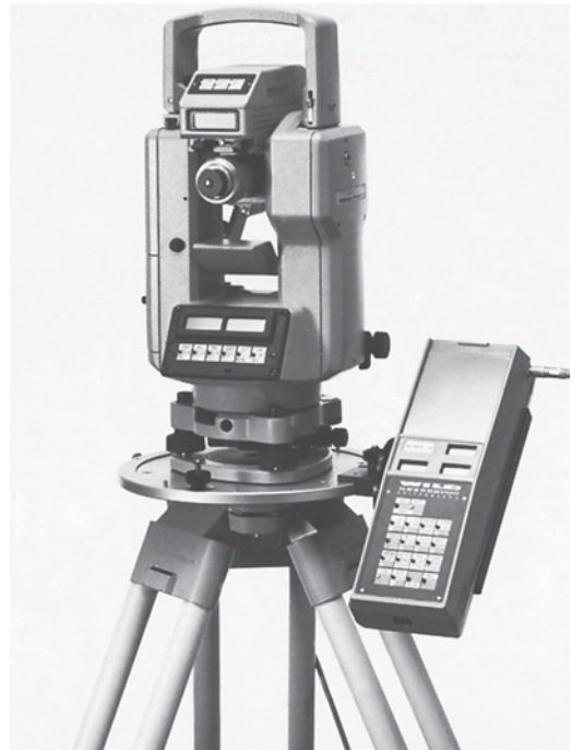
FIGURE 3-16 Wild T-1000 electronic theodolite, shown with D1 1000 Distomat EDM and the GRE 3 data collector
