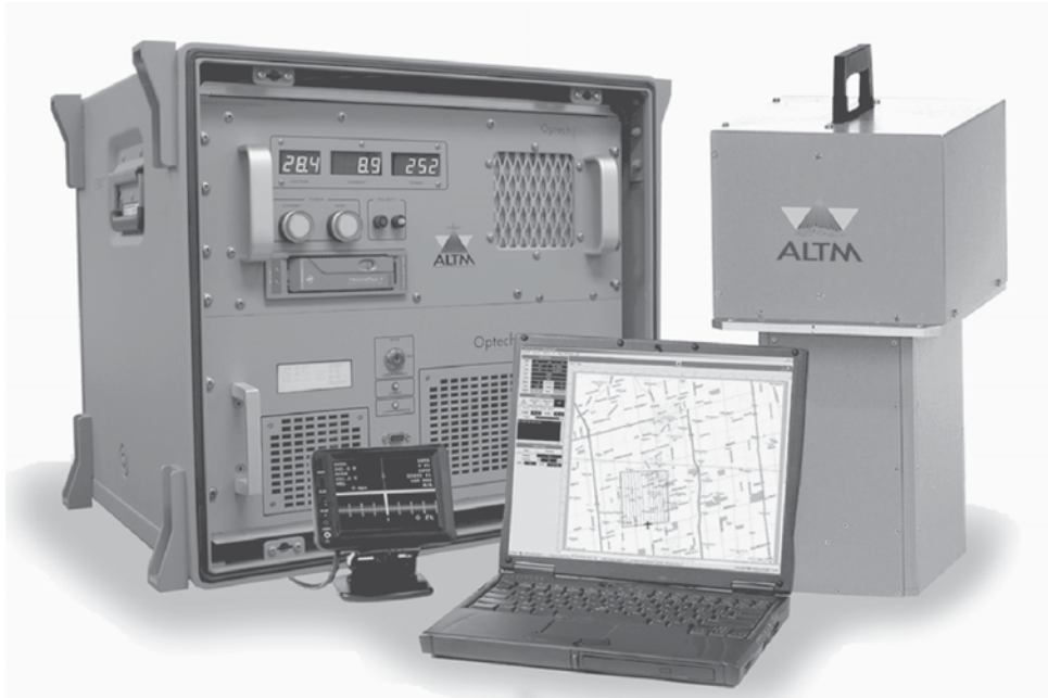
FIGURE 12-12 Complete ALTM 3100 system, including control rack, sensor, laptop computer (operator interface), and pilot display
