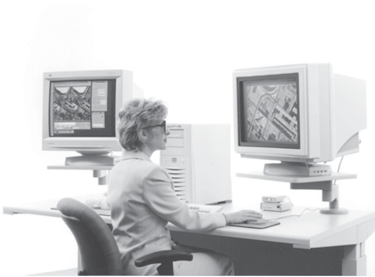
FIGURE 12-9 SOCET SET ® Windows NT workstation. This shot shows a human operator using the passive polarized viewing system, in this case the StereoGraphics ® Corporation ZScreen ® system: A polarizing bezel is placed and secured in front of an off-the-shelf, high-performance monitor. The operator wears passive, polarized spectacles
