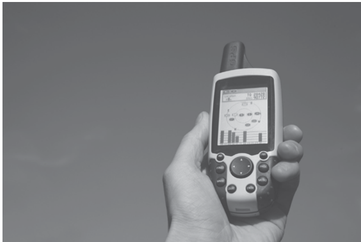
FIGURE 7-5 Garmin eMap handheld GPS receiver (accuracy: 15 m), used in navigation and GIS-type data location. It can be used with a DGPS radio beacon receiver to improve accuracy to within a few meters or less (Eimantas Buzas/Shutterstock)
