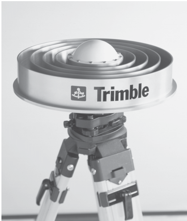
FIGURE 7-4 Geodetic-quality dual-frequency GPS receiver with a choke-ring antenna (Courtesy of Trimble)
