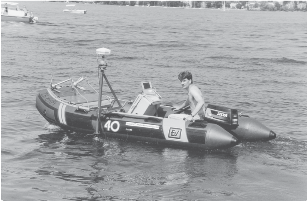
FIGURE 8-29 Leica GPS antenna and receiver on a small craft, providing positioning data for echosoundings in a differential kinematic mode. The data collector here is a notebook computer (Courtesy of Leica Geosystems Inc., Norcross, GA)
