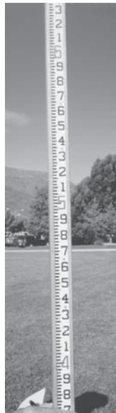
FIGURE 2-16 (a) Invar rod, also showing the footplate, which ensures a clearly defined rod position. (b) Philadelphia rod, which can be read directly by the instrument operator or the rod holder after the target has been set; Frisco rod, with two or three sliding sections having replaceable metal scales. (c) Metric rod; horizontal crosshair reading on 1.143 m
