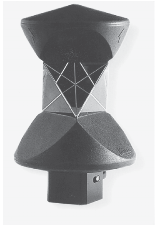
FIGURE 5-33 Leica 360° prism used with remote-controlled total stations and with automatic target recognition (ATR) total stations. ATR eliminates fine pointing and focusing. The 360° feature means that the prism is always facing the instrument (Courtesy of Leica Geosystems Inc.)
