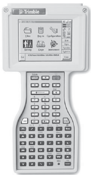
FIGURE 5-25 Trimble's TSCe data collector for use with robotic total stations and GPS receivers. When used with TDS Survey Pro Robotics software, this collector features real-time maps, 3D design stakeout, and interactive DTM with real-time cut-and-fill computations. When used with TDS Survey pro GPS software, this collector can be used for general GPS work, as well as for RTK measurements at centimeter-level accuracy
