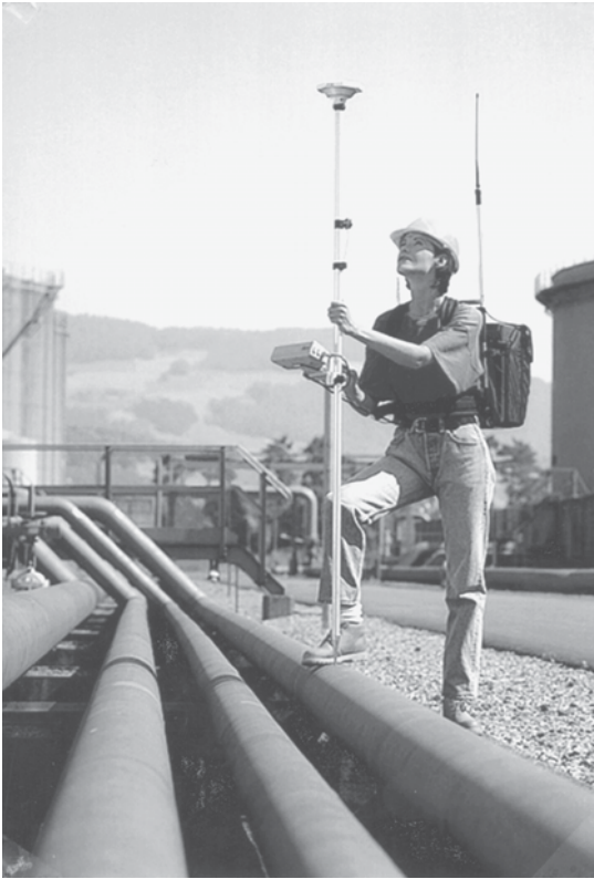
FIGURE 7-3 Leica SYS 300. System includes SR 9400 GPS single-frequency receiver, with AT 201 antenna, and CR333 controller which collects data and provides software for real-time GPS. It can provide the following accuracies: 10–20 mm + 2 ppm using differential carrier techniques; and 0.30–0.50 m using differential code measurements (Courtesy of Leica Geosystems Inc.)
