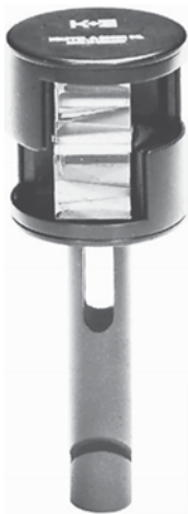
FIGURE 8-11 Double right-angle prism (Courtesy of Keuffel & Esser Company, Morristown, NJ)
