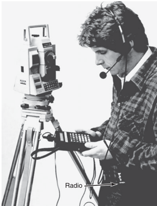
FIGURE 5-3 Total station with cable connected electronic field book. Also shown is a two way radio (2-mile range) with push-to-talk headset
