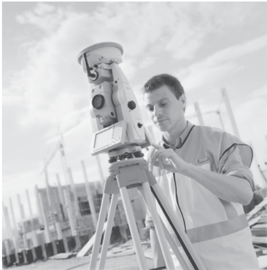
FIGURE 5-4 Leica Smart Station total station with integrated GPS
