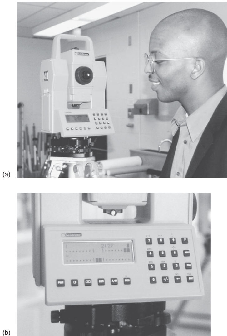
FIGURE 5-34 (a) Geodimeter 4400 Base Station. A total station equipped with servomotors controlling both the horizontal and vertical circle movements. It can be used alone as a conventional total station or as a robotic base station controlled by the remote positioning unit (RPU) operator. (b) Geodimeter keyboard showing in-process electronic leveling. Upper cursor can also be centered now by adjusting the third leveling screw
