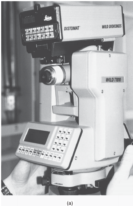
FIGURE 3-23 Distance measurement without reflectors. (a) Wild T1010 Electronic theodolite, together with an interfaced DIOR 3002S prismless EDM (angle accuracy is 3 seconds). (b) Illustrations of two possible uses for this technique. Upper: tunnel cross sections. Lower: profiling a difficult-access feature (Courtesy of Leica Geosystems Inc.)
