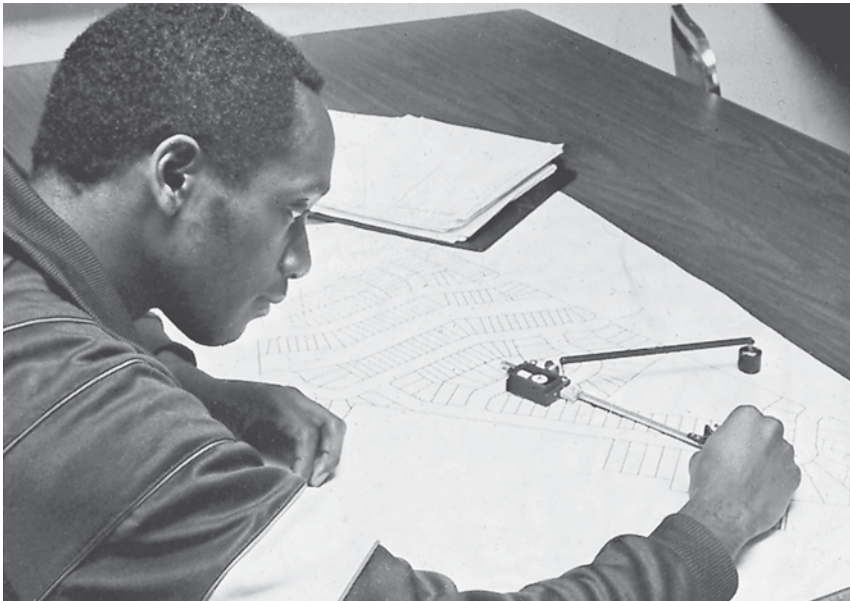
FIGURE 8-23 Area takeoff by polar planimeter
