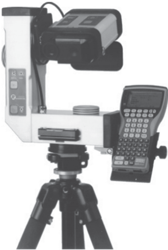
FIGURE 5-38 The Reflectorless Total Station is equipped with integrating distance measurement, angle encoding, and data collection
