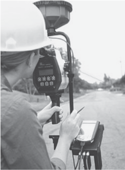
FIGURE 9-3 “Advantage Total Station” range finder. It can be equipped to measure horizontal distances, vertical distances, and angles from a baseline so that the surveyor can extend a GIS survey into areas where GPS signals are blocked
