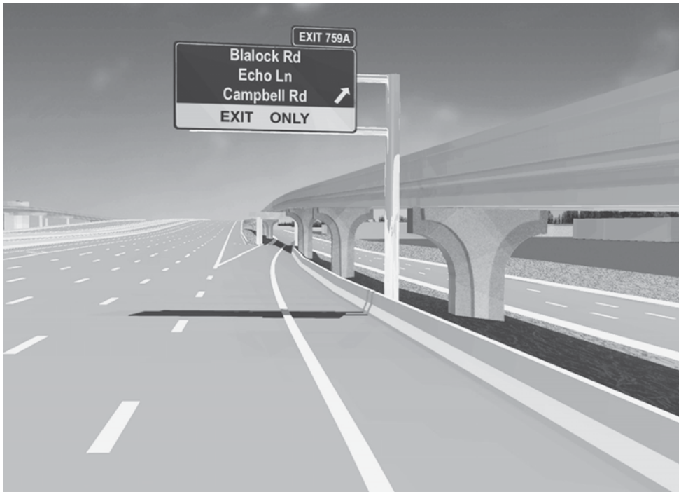
FIGURE 12-11 Highway design features such as signs and ramps can be developed using visualization software based on data extracted from LiDAR imaging
