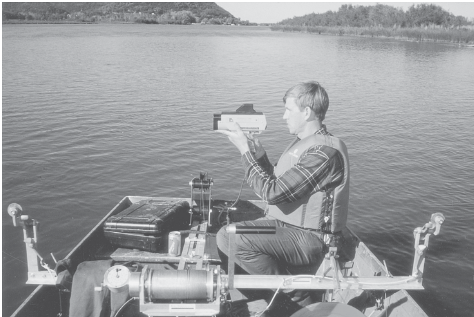
FIGURE 8-30 Prosurvey 1000 handheld survey laser: used (without prisms) to record distances and angles to survey stations. Shown here being used to determine river width in a hydrographic survey (Courtesy of Laser Atlanta, Norcross, GA)
