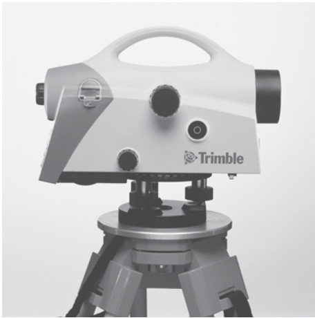
FIGURE 10-4 Precise level. Precise optical levels have accuracies in the range of 1.5 mm to 1.0 mm for 1 km two-way leveling depending on the instrument model and the type of leveling rod used. See also Figure 2-7
